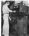
Purchased as surplus after war war was the S. S. Vetriche propeller test stand for use in maintenance shop. Good for up to 200 rpm, it checks control boxes and multiple registration.
